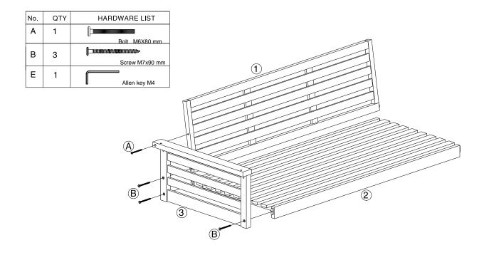
**STEP 2:** Use Bolt (A) and Screw (B) to attach The Right Arm (4) to the Back (1) and the Seat (2). Tighten all Screw using Allen Key (E).
