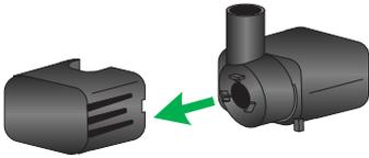
Filter cover can simply be pulled apart as shown.
