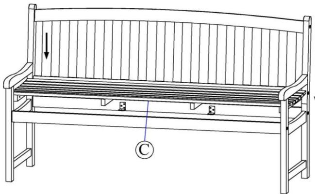
**3** **STEP 3:** Using the screw driver to tighten eight screws 4x30mm (3) to support under seat.
