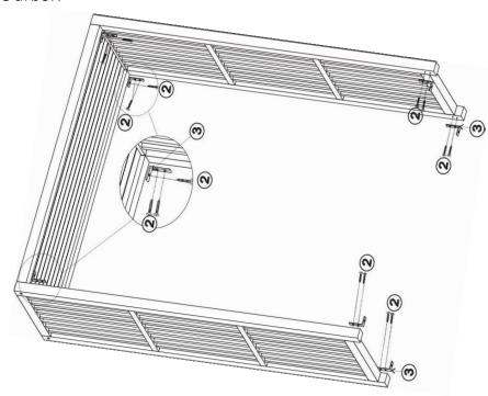
**Step 3**: Turn the Arbor upright. Put the Stake (4) through the Bracket hole and secure it in the ground by using the hammer (not provided )
