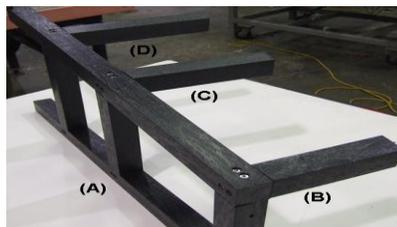
**Step 2:** Take one of the medium stringers (C) and place it at the middle set of holes. Screw it into place using two 2½" screws. Take one of the long stringers (D) and place it at the two bottom holes. Screw it into place the same way you did above.
