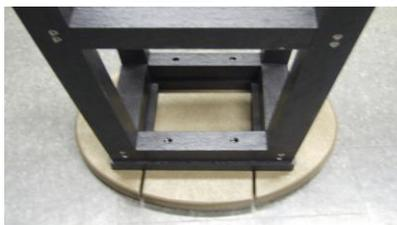
**Step 4:** Place the seat (E) upside down, with the square frame facing up. Place the legs on top of the frame, making sure the holes on the stringers are centered on the frame. Screw the stringers to the frame, using the remaining screws.
