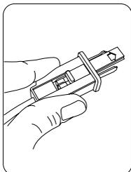
1. Grasp plug and remove from the receptacle or other outlet device. Do not unplug by pulling on the cord.
