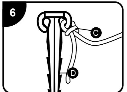
6 Using the loop at the end of the tether (C), fasten the tethers to the tether stakes (D).
