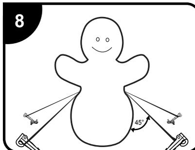
8 For maximum stability bring tether down to a 45-degree angle from the inflatable as shown in the illustration. In order to achieve this you may need to wrap the excess tether around the top of the stake.
