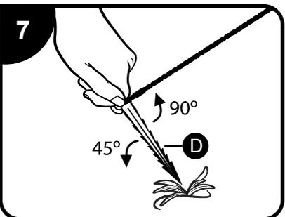
7 Drive the stakes (D) into ground at a 45-degree angle.
